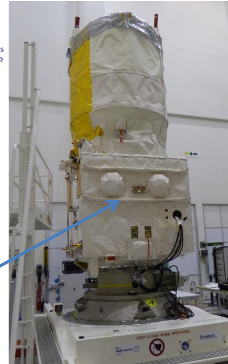
The ICS integrated on the Aeolus satellite
