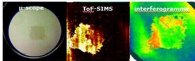
Analysis showing that the degradation of energy was due to LIC in the UV section (Aystorm/TEC-MMO)
