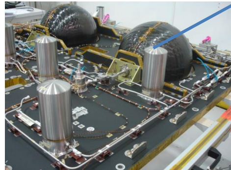
The In-Situ Cleaning System (ICS) developed to provide O 2 to the UV high emission path optics and prevent LIC (Airbus)
