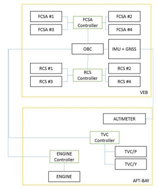
Figure 10 : Flight Control architecture overview
