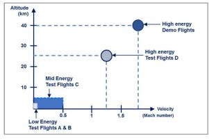
Figure 12 : Test & Demo Flights – some features
