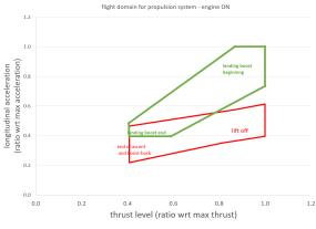
Figure 5 : Longitudinal acceleration vs Thrust flight domain
