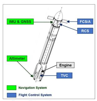
Figure 8 : Flight control - reentry configuration
