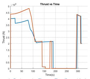
Figure 3 : Rocket engine Thrust vs Time (Bottom) for 2 different flight classes #1(red) and #2(blue)
