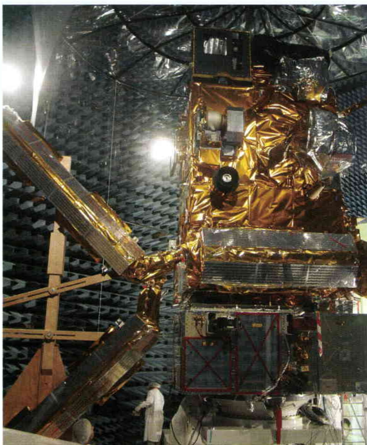
MetOp-1 in the anechoic chamber at Intespace (F)
