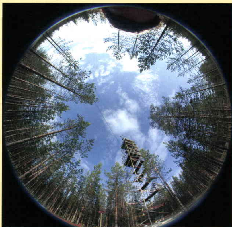
The experimental setup during the ESA SIFLEX campaign which took place above the Arctic Circle, in Sodankylä, Finland. Observations of solar-induced fluorescence were made from the top of a 20 m tower overlooking the boreal forest canopy.
