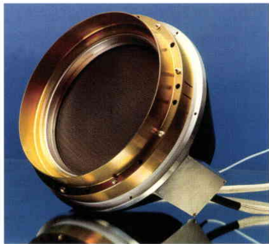
RIT-XT Development Model Thruster during operation in the vacuum facility at Giessen (D)
